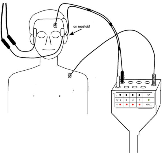
to Thymatron System IV EEG/ECG/EMG
